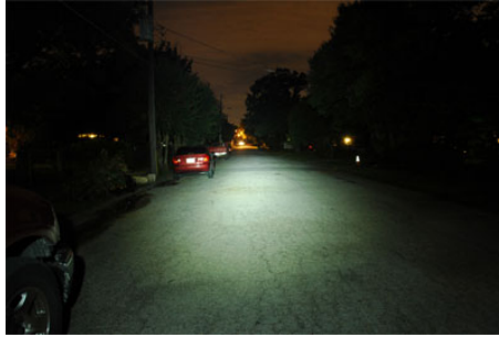
The same street illuminated with the MUL-15-4V, easily reaching distances of 90' in length and 70' in width.
